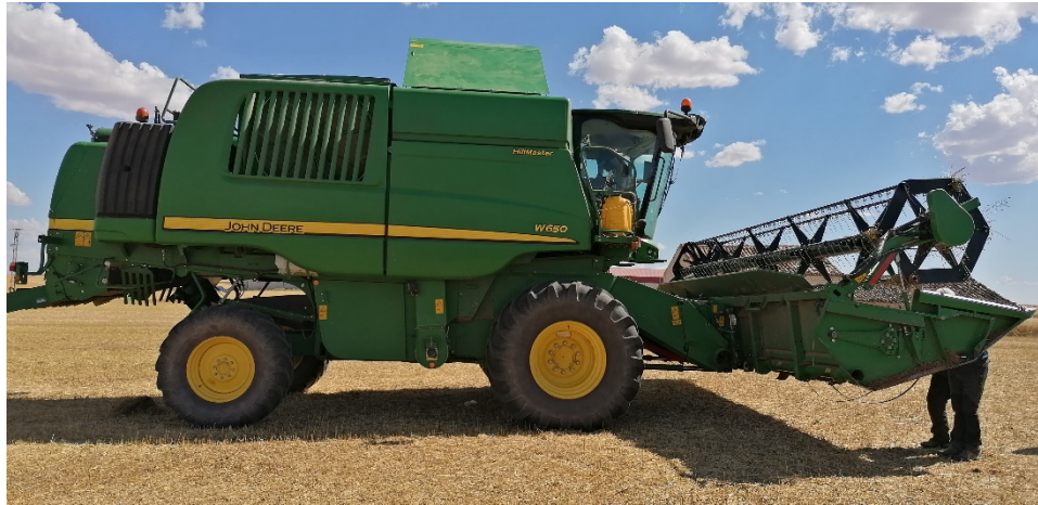
Figure 2. John Deere W650 combine harvester equipped with a cereal header.
